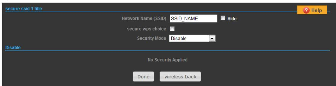
The screenshot shows the 'secure ssid 1 title' security setup screen. It includes: 'Network Name (SSID)' (SSID\_NAME), a 'Hide' checkbox, 'secure wps choice' (checkbox), 'Security Mode' (Disable), and a 'Disable' link. At the bottom, it says 'No Security Applied' and has 'Done' and 'wireless back' buttons.
