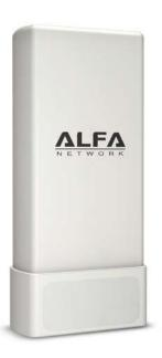
WISP-2 is a Low-Cost 802.11n outdoor AP/CPE operating in 2.4GHz band that is also compliant with the standard IEEE 802.11b/g.
