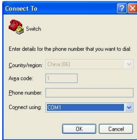
Figure 19 Selecting the Communication Port in Use
